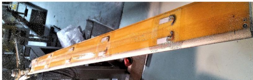
Figure 4. Embedded array of deformation sensors and wiring
