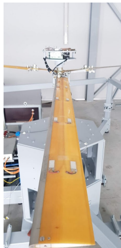
Figure 1. Blade with embedded piezo film sensors and measurement system
